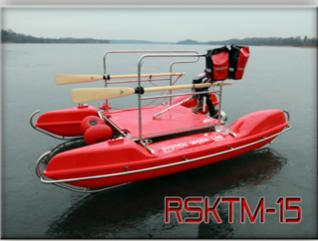
The RSKTM-15<sup>®</sup> water - ice system is all year round mobile rescue water motorboat for evacuation operations in water and ice conditions, where the main difficulty in reaching the injured person is ice breaking and drifting or long waterways between land and ice.
